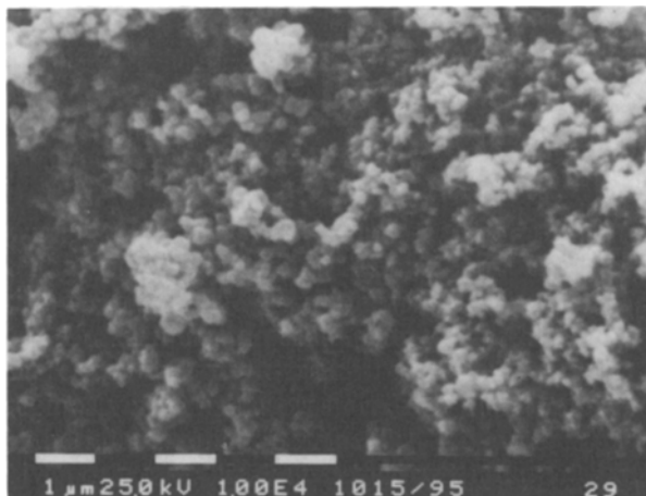
Fig. 8 Scanning electron micrograph of a manganate showing the end of the first mass loss in a 5% H 2 /95% N 2 atmosphere at 460°C
